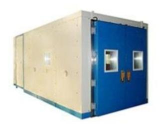
Execution and meet the standards: GB / T2423.3 (IEC60068-2-78), GB / T2423.4 (IEC60068-2-30), GB / T2423.34 (IEC60068-2-38), GB / T2423.40 (IEC60068-2-66) / ISO16750, JESD22, GB / T 14710: 2009, GB / T 13543. Uses: The <u>walk in chamber</u> <u>Walk-In High and low temperature test Room</u> is Suitable for the test of large components.
