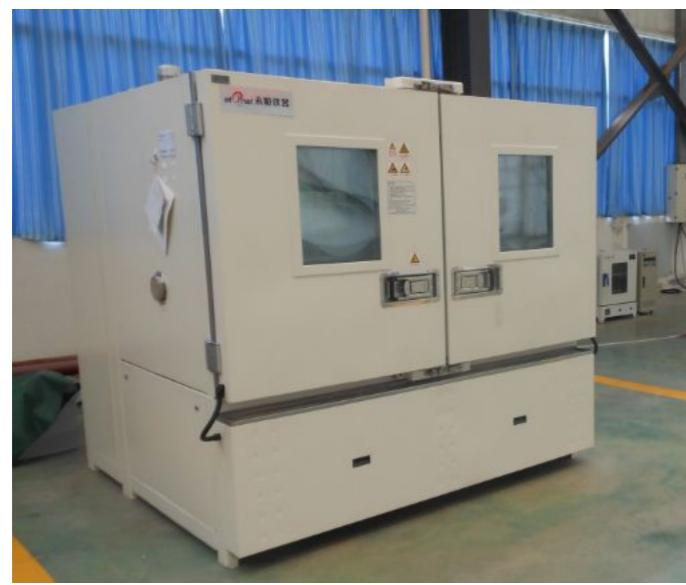
Execution and meet the standards: IEC60068-3-5, IEC60068-3-6 Purpose: To achieve rapid temperature change, find product design defects and process issues
